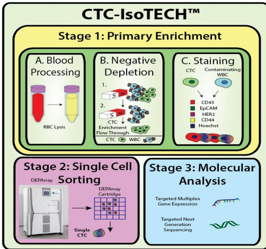
**Figure 1.** CTC-isoTECH platform description. Stage 1 includes whole blood processing, a negative immunomagnetic depletion of unwanted white blood cells followed by staining of the enriched cells. Stage 2 consists of single cell sorting by the DEPArray and, lastly, Stage 3 provides for molecular analysis of the single cells including gene expression analysis and next generation sequencing.
